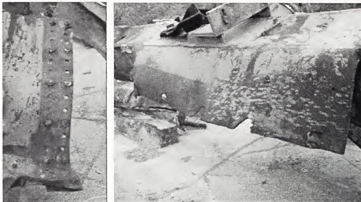
Figure 5–11. Typical bolt bearing shear failures of spandrel connections.
